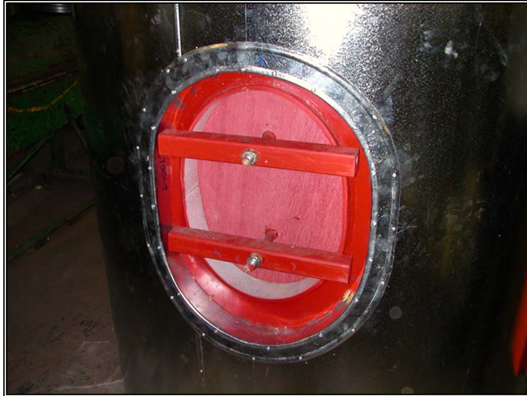
Finished metalwork around inspection plate
